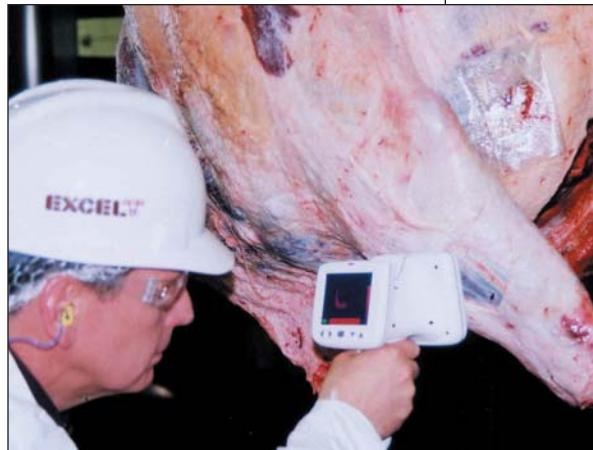
*Emerging “pre-intervention” technologies, such as this prototype of a handheld scanner to detect fecal contamination being tested by Excel Corp., are being introduced with increasing frequency. (Photo courtesy of eMerge Interactive)*
